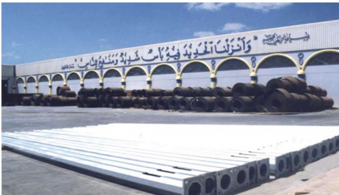
All galvanized products are packed and bundled with wooden spacers before delivery to customers
